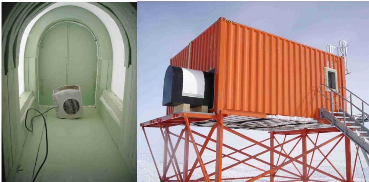
Interior of the shield with the heater HAMSTRAD shelter with the shield attached to it (on the left)
