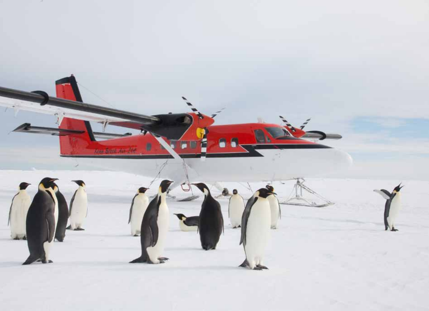
Emperor penguins surround the aircraft just arrived. The DHC-6/300 Twin Otter, equipped with skis, is particularly suited for intracontinental flights, e.g. from the coast to Dome-C. It carries one ton load or 8 passengers.
