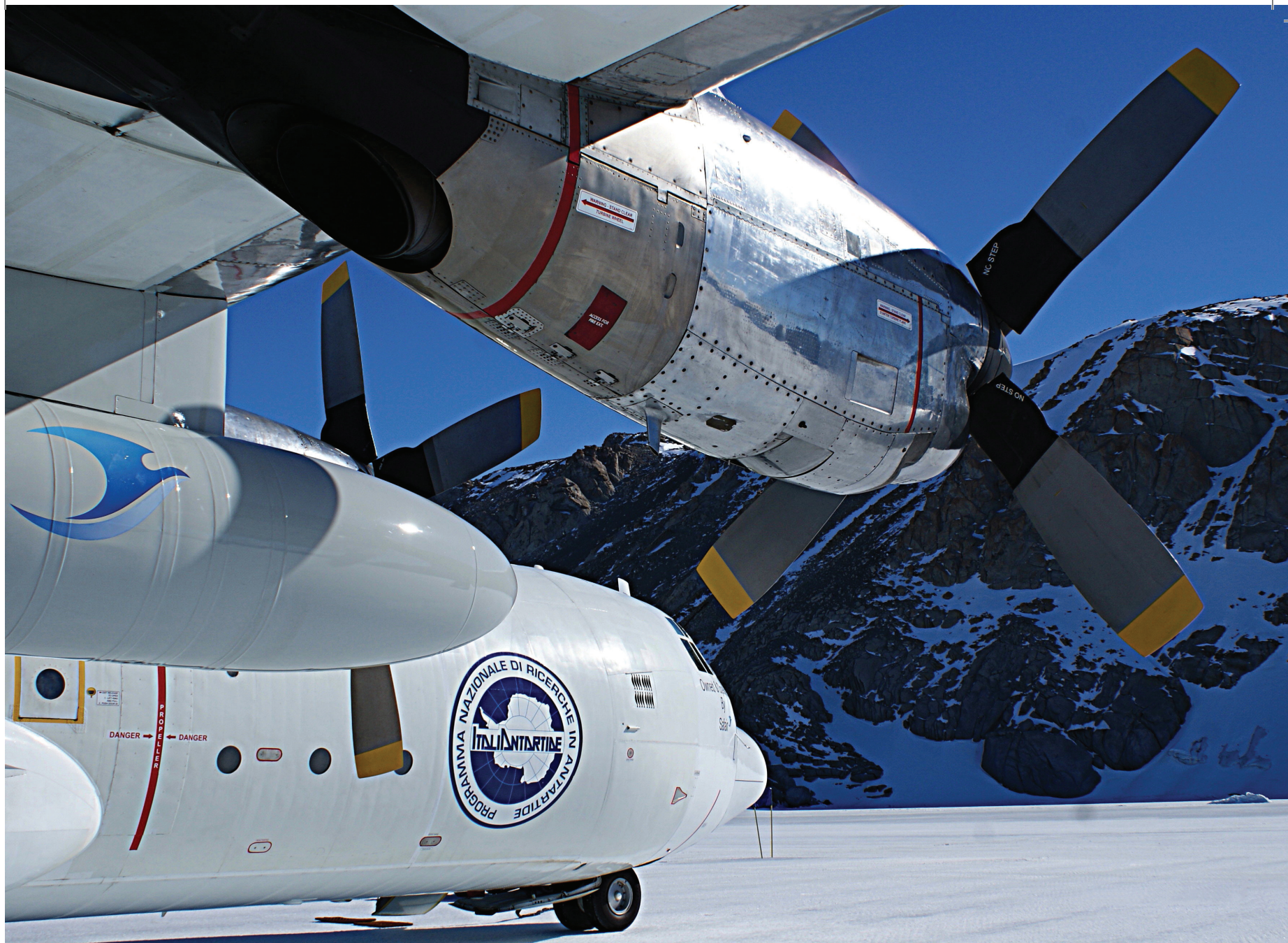
The L-100/30 is a commercial version of the well-known C-130, which is the military version of the Hercules' family. It carries a load of 11 tons or 45 passenger from New Zealand to Victoria Land in 8 hours.
